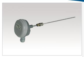
Technical data: NTC 10-KB element sensor R 1/4" thread mounting Ø 4 mm x 200 mm stem cable entry M16 -50...+120 °C range ±0.5 °C (at 25 °C) accuracy about 2.5 s time constant PN16 pressure rating protection class IP54, cable entry or stem down
